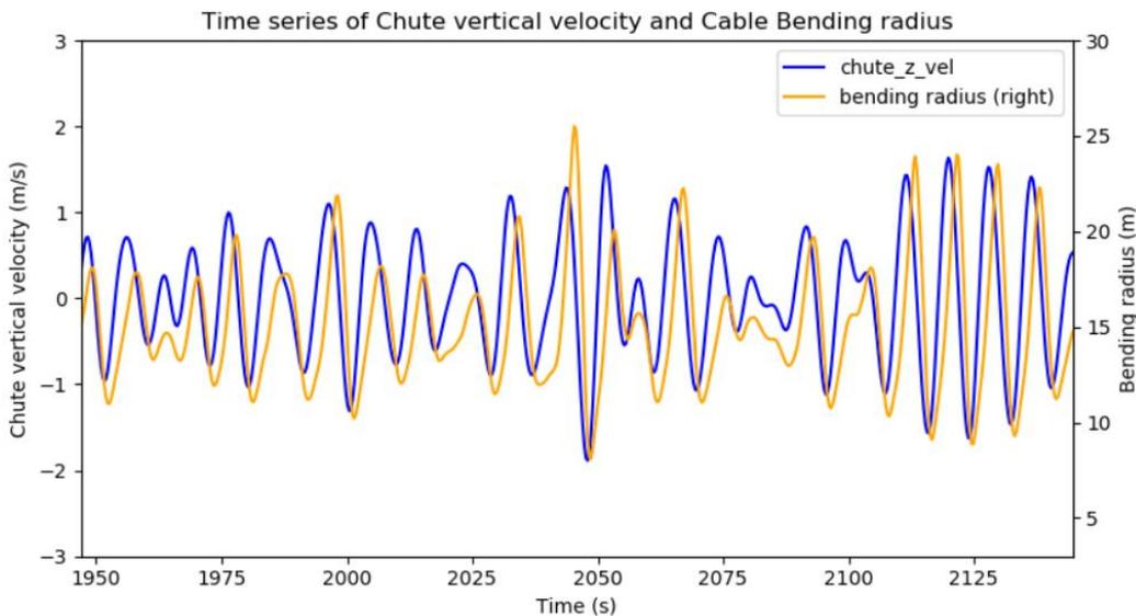
Figure 4: Time series of chute velocity (left axis) and cable bending at touch down point (right axis) from simulation in Orcaflex. (source: Havkonsult)
