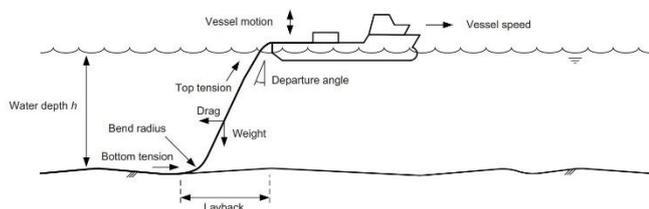
Figure 1: Free cable lay operation terminology (source: DNV GL)
