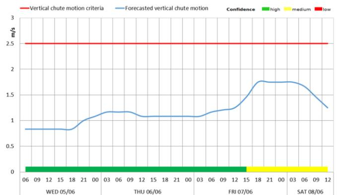
Figure 3: Typical vertical wheel/chute motion forecast received every sixed hour. The graph is based on vessel RAOs and onsite weather forecast. It can be seen from the forecasted that chute motion will stay well below allowed chute motion for the next few days (source: Havkonsult)
